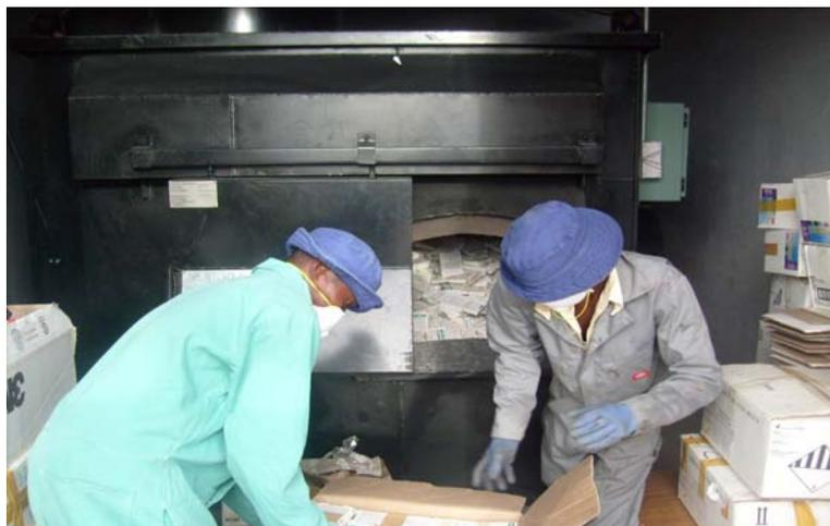
**Empty insecticide sachets are packed into the incinerator for disposal.**
